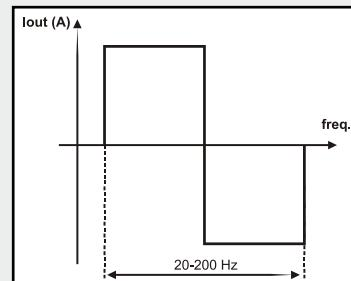
**BALANCE:** Allows you to reduce the amount of current for cleaning to the advantage of that for welding (just think that generators normally use 50% of the power for cleaning and 50% for welding); in welders the ratio is 35% -65%.
