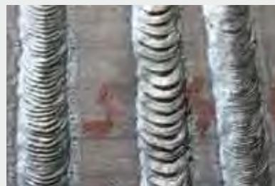
**Fig.B** Appearance of deposits made with cellulosic electrode
