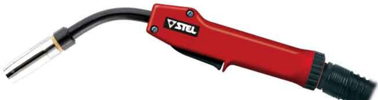
The torch for Mig / Mag Welding is used when high productivity is required and a suitable flexibility of use. With this technology you can weld steel is austenitic and ferritic alloys of light metals (Al and Mg), copper alloys, nickel alloys and titanium alloys.
